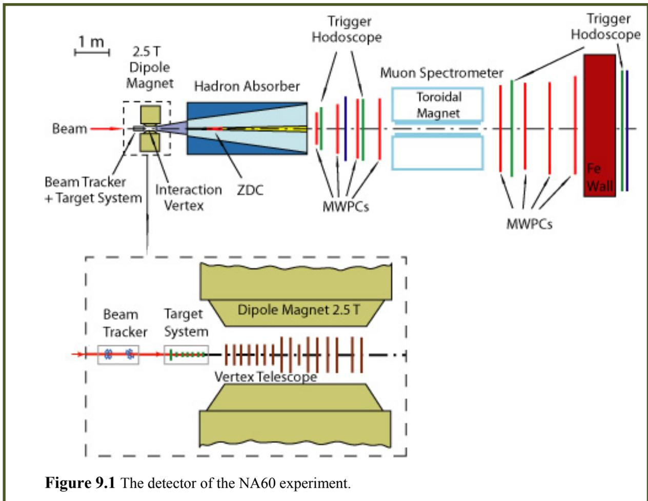
**Figure 9.1** The detector of the NA60 experiment.
